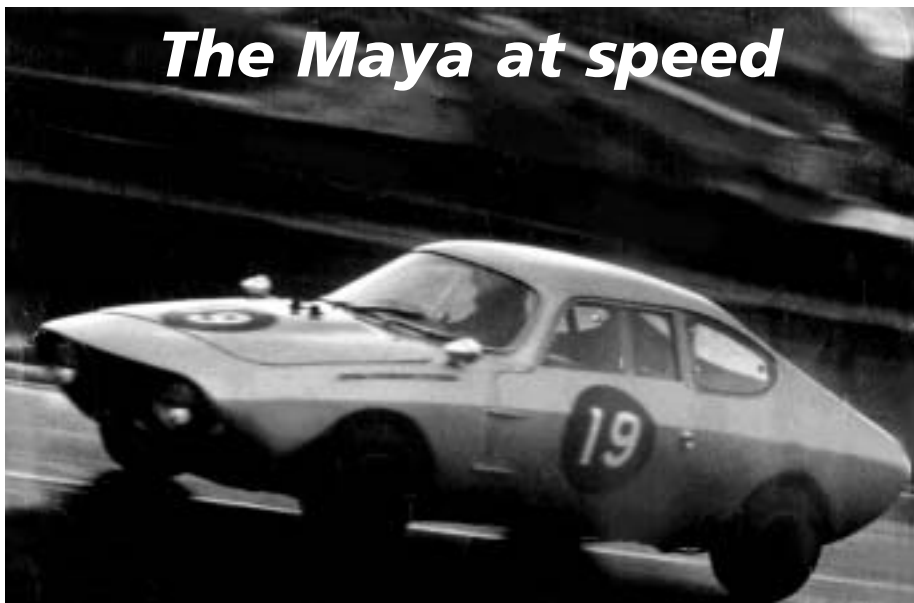
Photographed at Brands Hatch in March 1967 on its way to a class win. Note the 46 IDA trumpets on the bonnet! Then reverted to a 45 DCOE.
